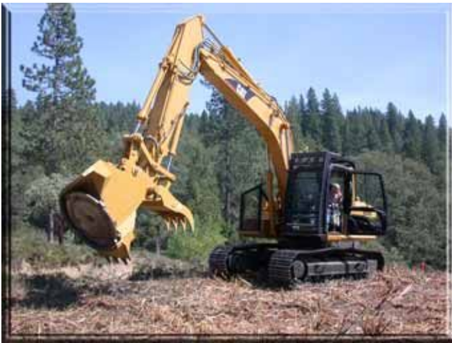
Figure 77: A masticator mulching a brush field in the wildland urban interface located in the Hume District-Sequoia National Forest. Photograph by Timothy Walsh.
