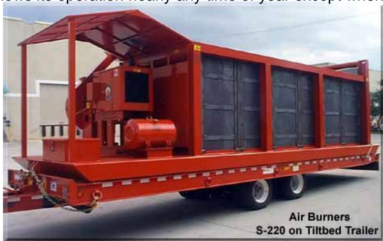
Figure 74: Example of a medium sized Air Curtain Destructor mounted on a lowboy trailer. Photo from the AirburnerWebsite.
