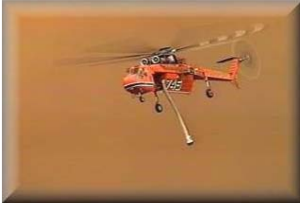
Figure 18: Type one helitanker preparing to drop water on the Manter Fire.
